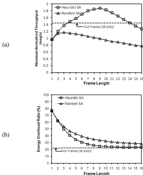
Fig. 6 Performance under maximum traffic load: (a) maximum normalized throughput, (b) energy overhead ratio.
