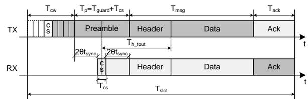
Fig. 3. Channel access scheme of RF-TDMA protocols.
