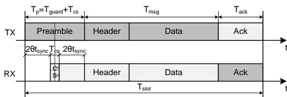
Fig. 1. Channel access scheme of FF-TDMA protocol.
