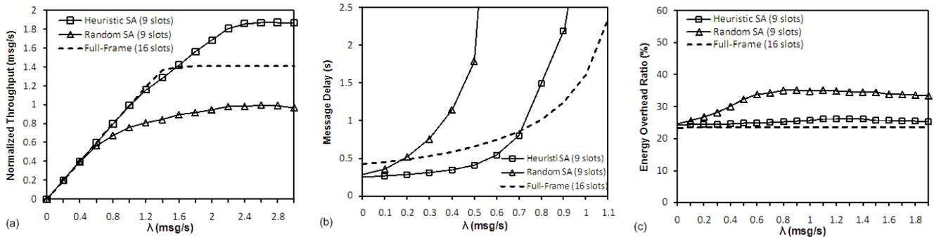
Fig. 5 Performance under varying traffic load: (a) normalized throughput, (b) message delay, (c) energy overhead ratio.
