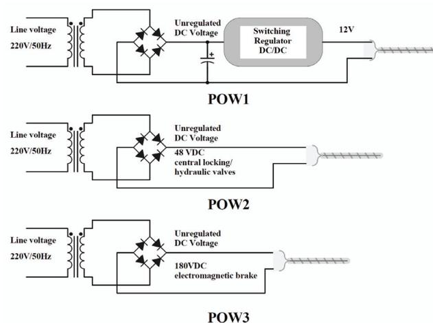
Fig. 1. Typical voltage values of the lift system
