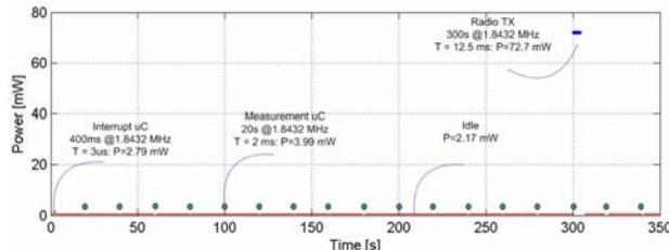
Fig 7. Power consumption for our system during a period data-sampling and communication time
