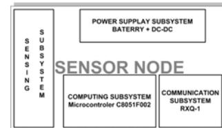
Fig 1. Block structure sensor node
