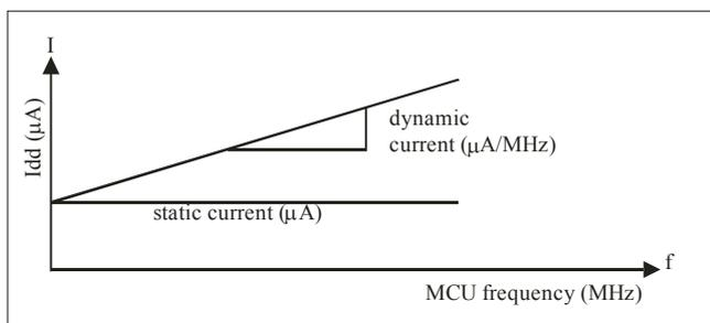
Fig. 2. Dynamic versus static current
