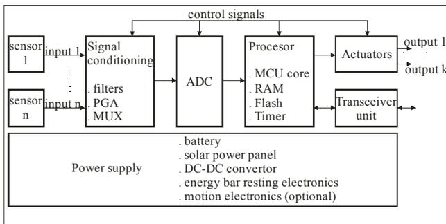
Fig. 1. System architecture of a typical wireless sensor node
