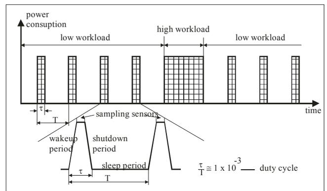
Fig 3 Two phases of SN's operation
