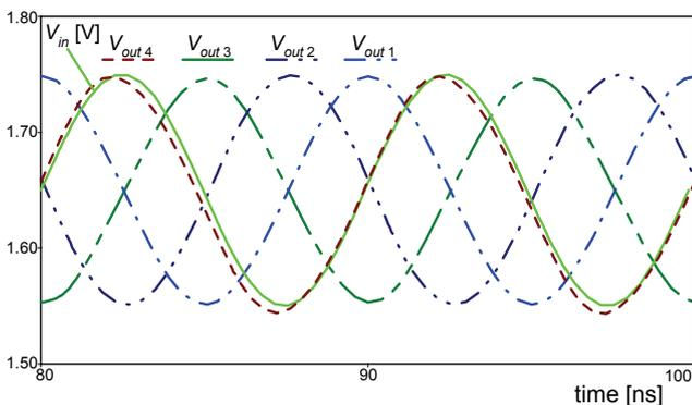
Fig. 9. Waveform of signals on outputs of all-pass filters
