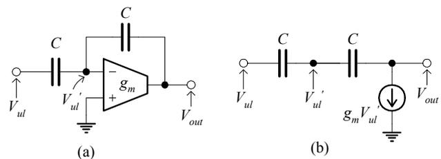
Fig. 1. (a) Scheme of the all-pass filter, (b) electrical model
