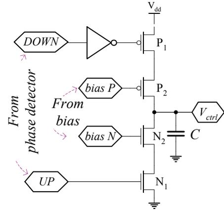
Fig. 7. Charge pump with loop filter
