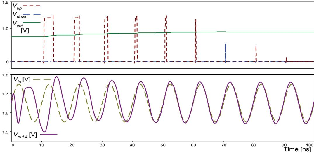
Fig. 8. DLL for analog signal transient simulation waveform
