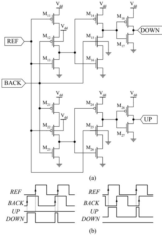
Fig. 6. (a) Scheme of dynamic phase detector, (b) signals waveforms
