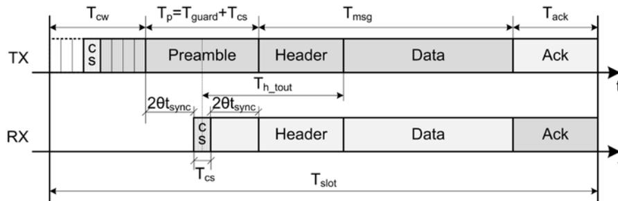
Figure 4. Channel access scheme of hybrid TDMA/CSMA protocols.
