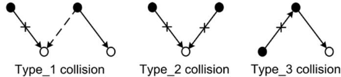
Figure 3. Types of collisions in multi-hop wireless networks.
