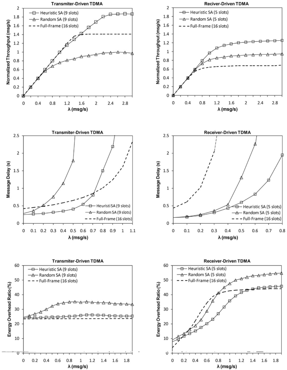
Figure 8. Performancemetrics of TDMA-based protocols under maximum traffic load: (a) and (b) maximum normalized throughput; (c) and (d) energy overhead ratio.
