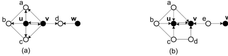
**Figure 6. Reduced-frame TDMA slot assignment: (a) transmitter-driven slot assignment; (b) receiver-driven slot assignment.**
