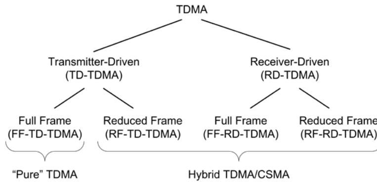
Figure 1 Classification of TDMA-based protocols.
