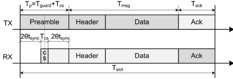
Figure 2. Channel access scheme of full-frame transmitter-driven TDMA protocol.
