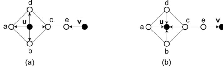
Figure 5. Full-frame TDMA slot assignment: (a) transmitter-driven slot assignment; (b) receiver-driven slot assignment.
