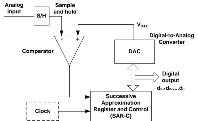
Fig. 1. Successive approximation analog-to-digital converter.
