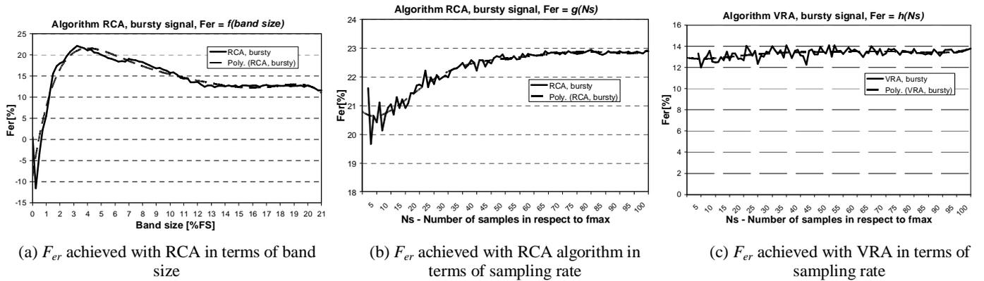
Fig. 6. Energy reduction factor ( $F_{er}$ ) for bursty signal.
