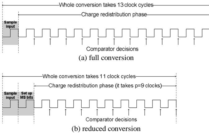
Fig. 2. Timing diagram of SAR-ADC.
