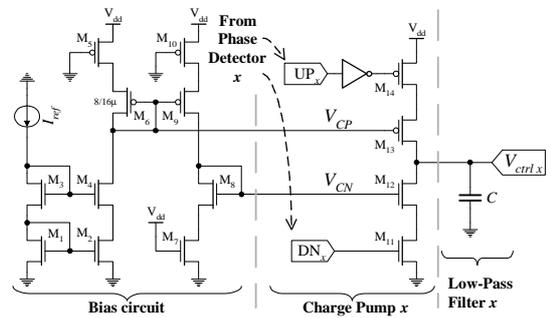
Fig. 7. Current pump and loop filter
