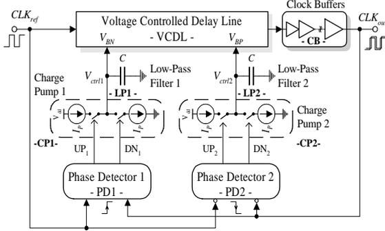
Fig. 1. DLL's architecture with double edges synchronization
