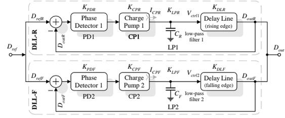
Fig. 2. Equivalent model of DLL-DES.
