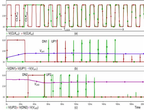
Fig. 8. Simulation of DLL with Double Edges Synchronization
