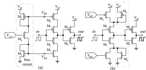
Fig. 3. Modified current starved delay element
