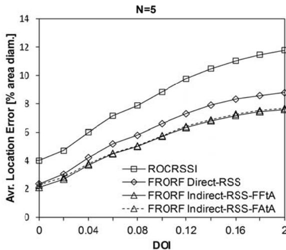
**Fig. 12.** Localization error vs. degree of radio propagation irregularity for ROCRSSI and FRORF algorithms.
