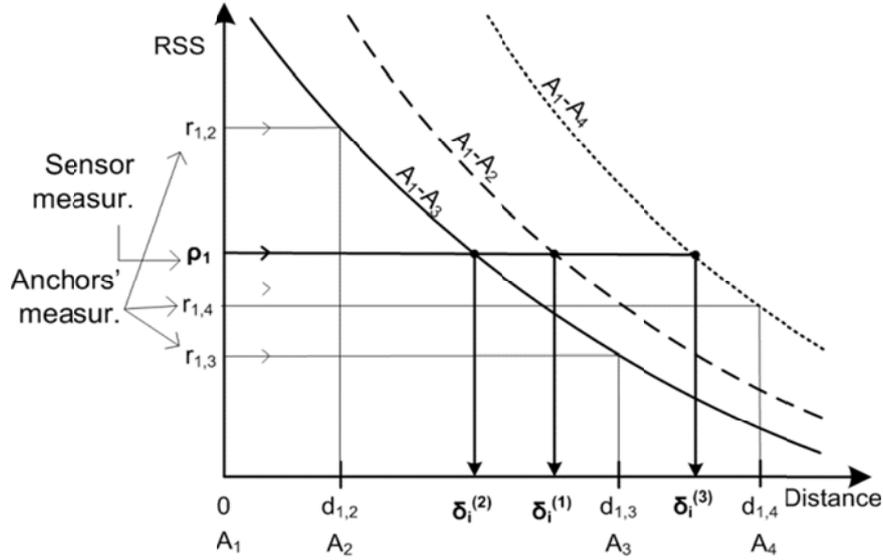
**Fig. 8.** Possible estimated distances of sensor  $S$  from anchor  $A_i$  due to various radio propagation characteristics in different direction of propagation.
