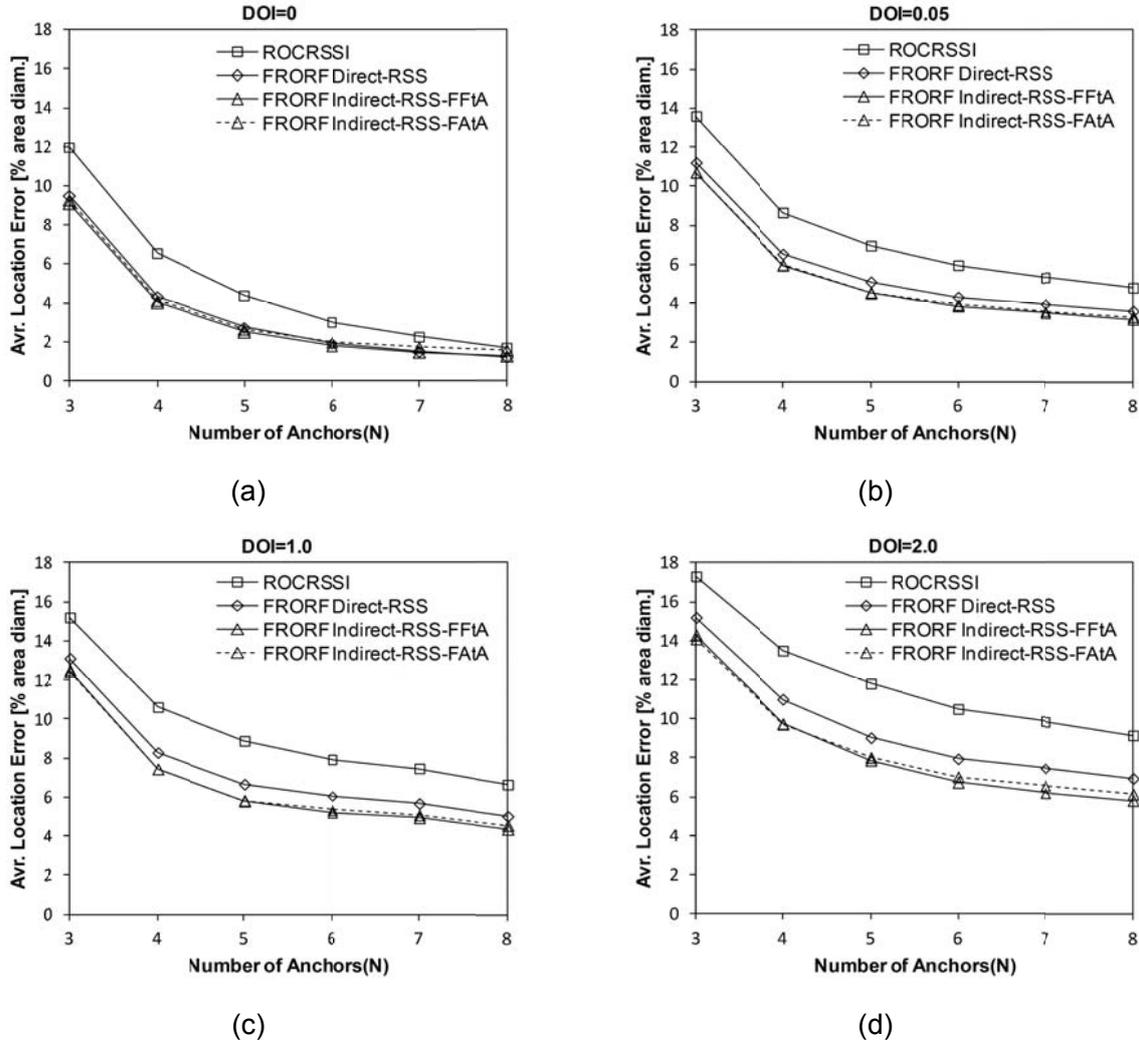
**Fig. 11.** Localization error vs. number of anchors for: (a)  $DOI = 0$ ; (b)  $DOI = 0.05$ ; (c)  $DOI = 0.1$ ; (d)  $DOI = 0.2$ .
