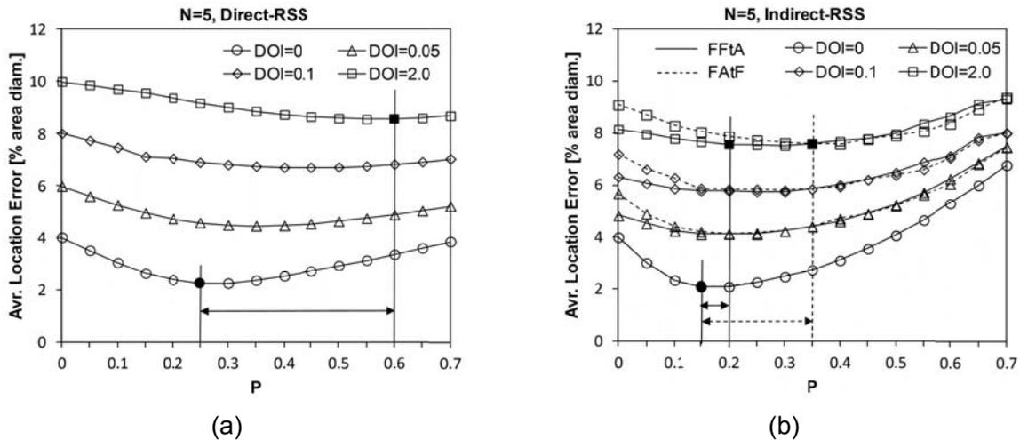
Fig. 10. Localization error vs. level of fuzzification ( $P$ ) for four different degrees of radio propagation irregularity (DOI): (a) FRORF, Direct-RSS fuzzification; (b) FRORF, Indirect-RSS fuzzification.
